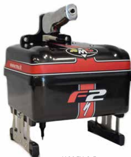
MODELLO F2 AREA DI LAVORO 100X100 MM F2 MODEL - WORKING AREA 100X100 MM
